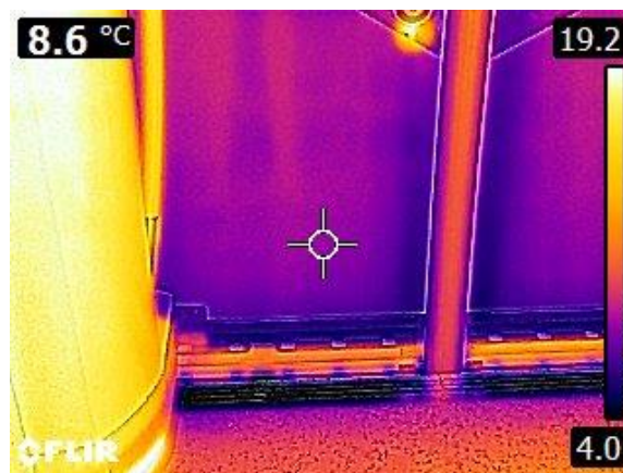
Figure 69 - Indoor side of doors surface temperatures (around -1°C outdoor temperature)
