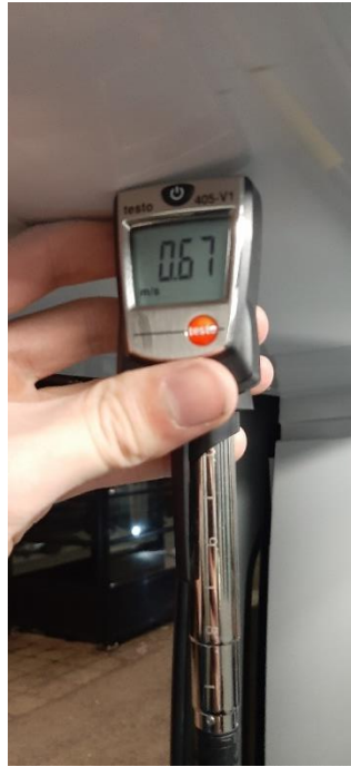
Figure 71 - Measurement at upper vertical section of the train door. Outdoor temperature around 0°C.
