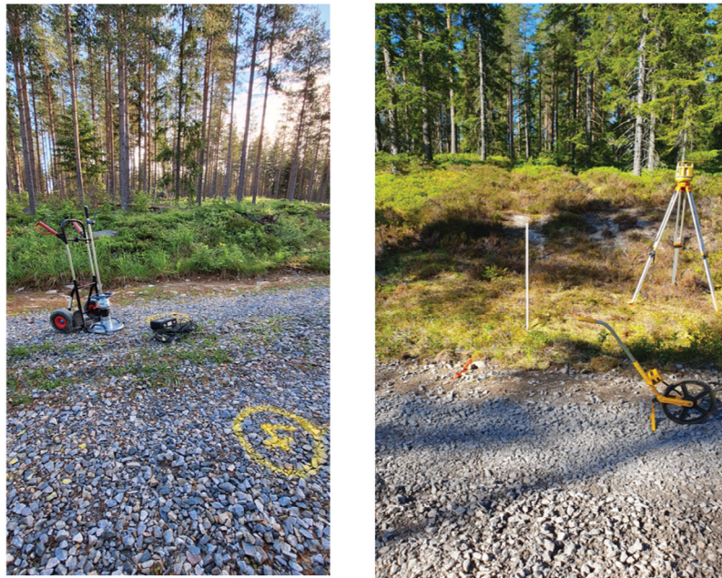
Figure 7. The post-construction measurements before and after traffic and weather impacts of the road sections. Photos: Andreas Waldemarson, VTI.
