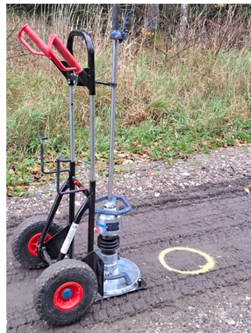
Fig. 1. The lightweight deflectometer used in the project. Photo: Dina Kuttah, VTI.
