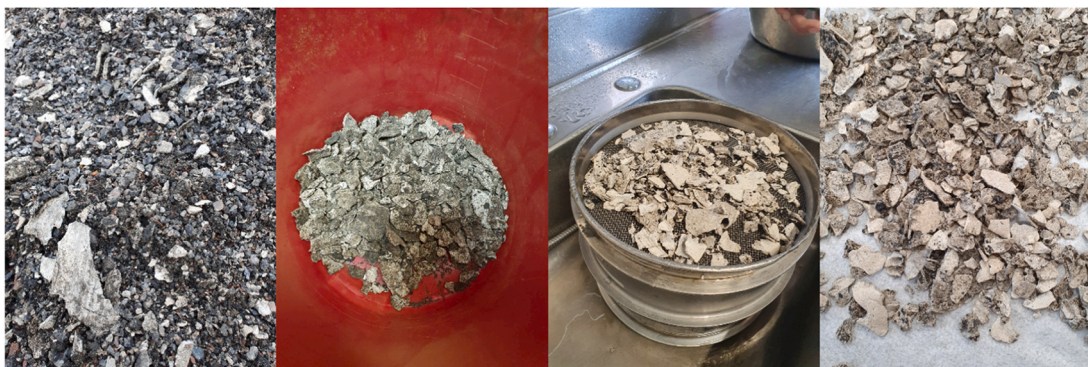
Fig. 1. From left to right: (1) Recovered MM as collected, containing a mixture of thermoplastic road marking, asphalt residue, gravel, and dust; (2) material after the initial sieving step; (3) material during the washing process; and (4) cleaned and processed material following sieving, manual sorting, and washing.
