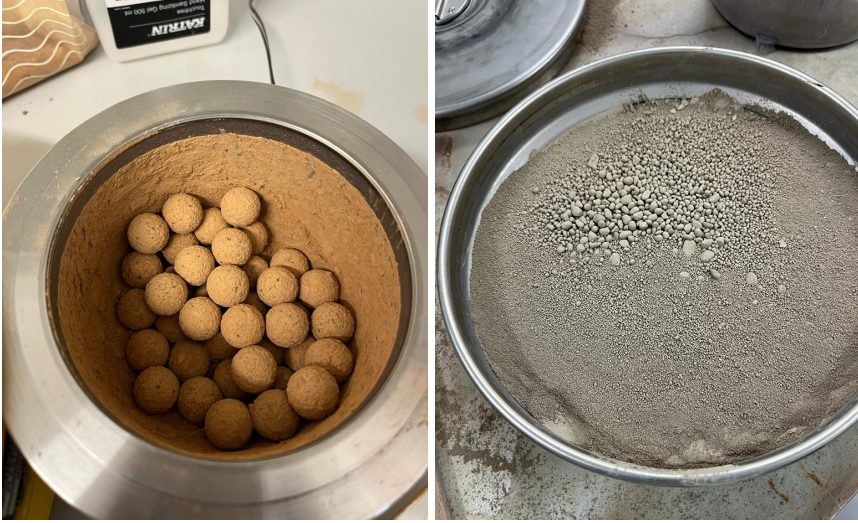
(a) Agglomerations after milling calcined clay
