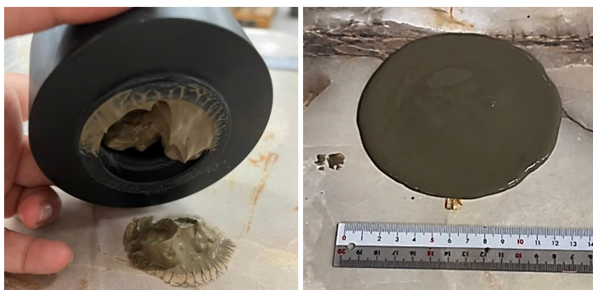
(a) Stiffer mix as observed with mixed clay particle sizes (b) Improved flows observed with controlled clay particle sizes
