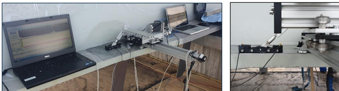
Figure 12. Field application of TOFD in LifeExt-2, with the new larger manipulator.
