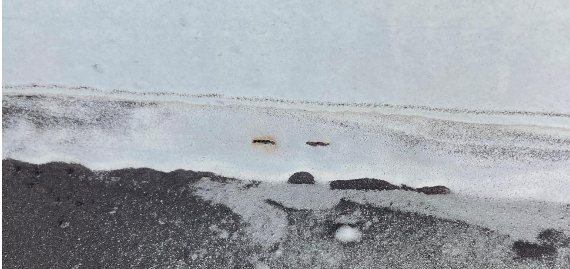
Figure 17. Centre cracks found in the main weld holding the lower flange to the web.
