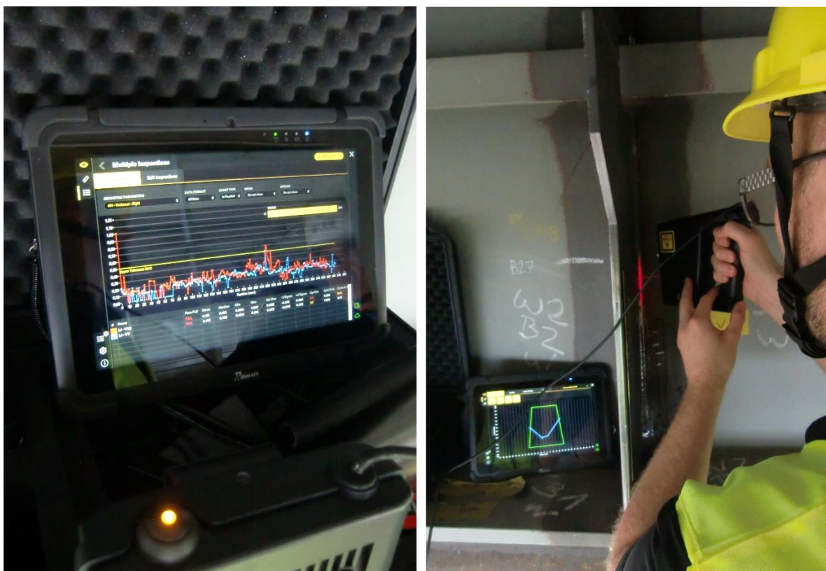
Figure 19. Laser scanning of weld of vertical reinforcement in conjunction with HFMI-treatment. This was done with the Wintertia Flex system both before and after HFMI-treatment, which gave precise measurements of the whole HFMI groove.
