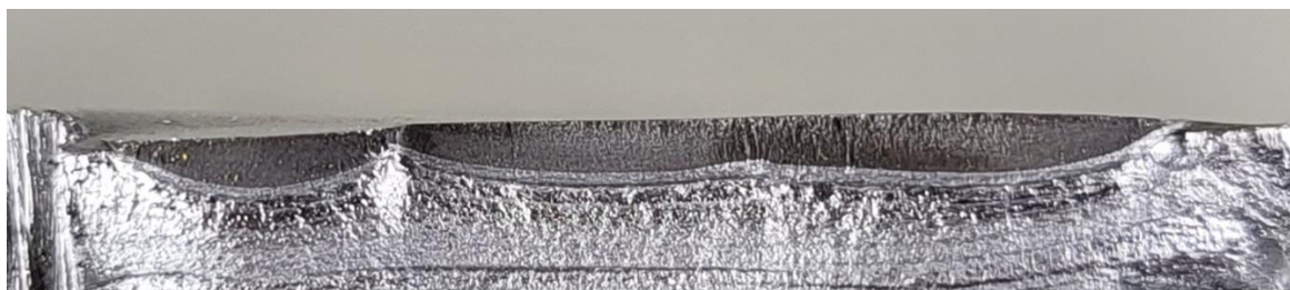
Figure 9. Cut out from cope-hole specimen for verification of TOFD accuracy. Multiple crack-starts (black areas) visible in the upper part of the image (the image is a cross-section from “the inside” of the cope-hole, where the fatigue cracks have initiated in the weld toe).
