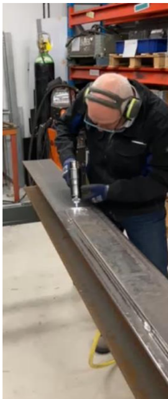
Figure 5. HFMI-treated end section of the cover plate weld for the HEA-beam (left), and the fatigue results (right).
