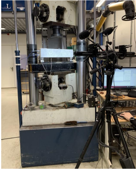
DIC system set up
