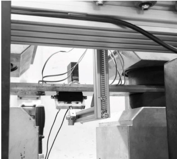
Manipulator developed for test specimen type 2, non-load carrying transverse gusset plate
