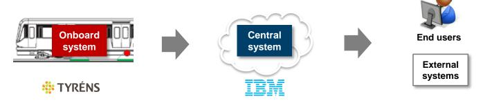
The **onboard system** is mounted on the trains and consists or microphones and other equipment to detect the condition of the track. The **central system** is running in IBM Cloud and contains components to store and present track data, and generate alerts
