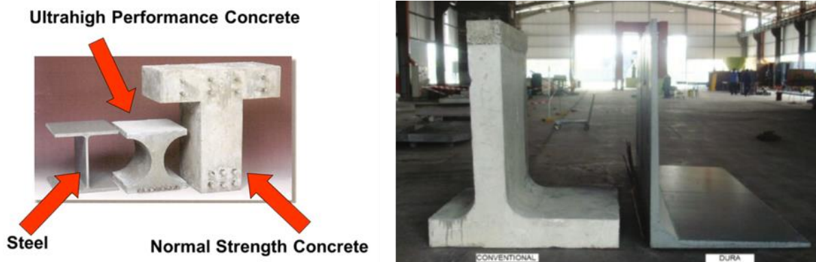
Figure 1 Comparison between elements having approximately the same load bearing capacity: (left) steel, UHPC and OPC and (right) OPC and UHPC.
