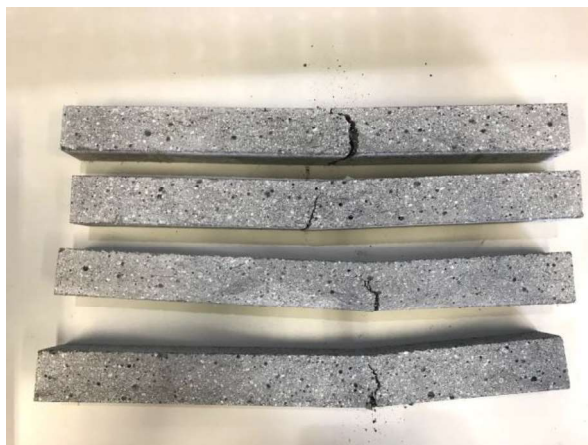
Figure 3-3 Samples after flexural testing, CBI FA 2,5% .
