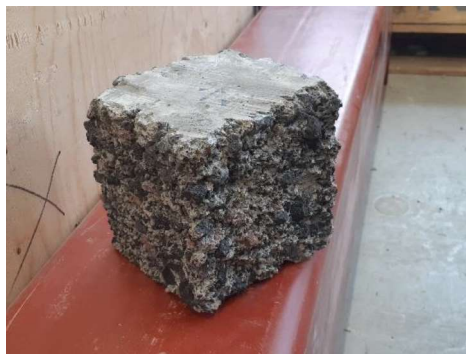
Figure 4-3 Scalled (water jetted) cube
