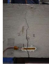
Figure 4-173: Macro-cracking of NSC from FEM (left) and full-scale test (right).
