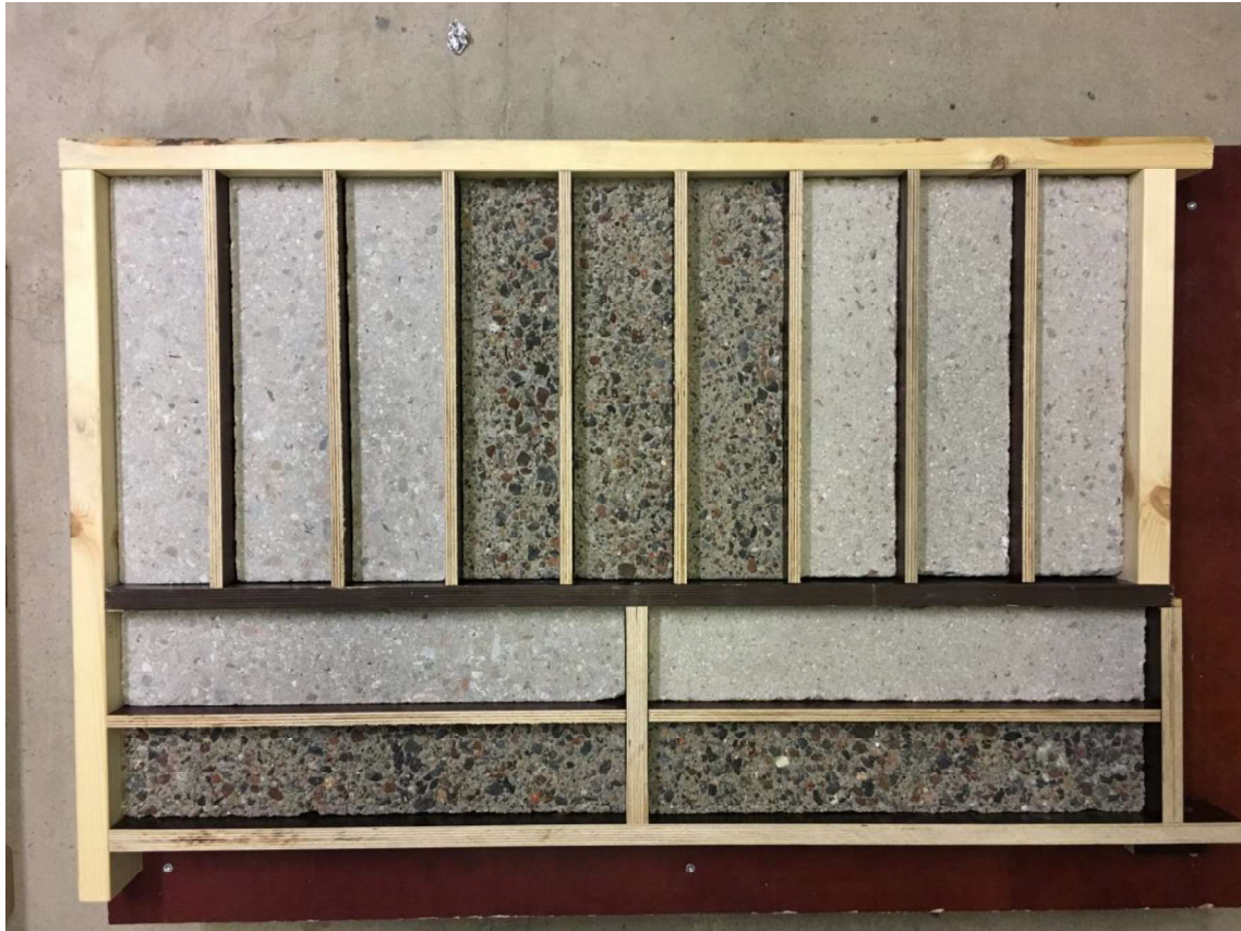
Figure 3-13 Form for overlay with different surface treatment of reference concrete. Tests: Shear, 4-point bending
