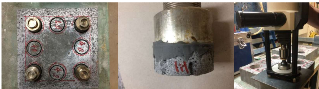
Figure 3-16 a) picture from above before pulling b) pulled specimen c) Pulling machine
