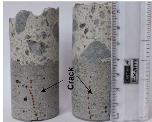
Figure 4-12: Cracks depth of composite concrete
