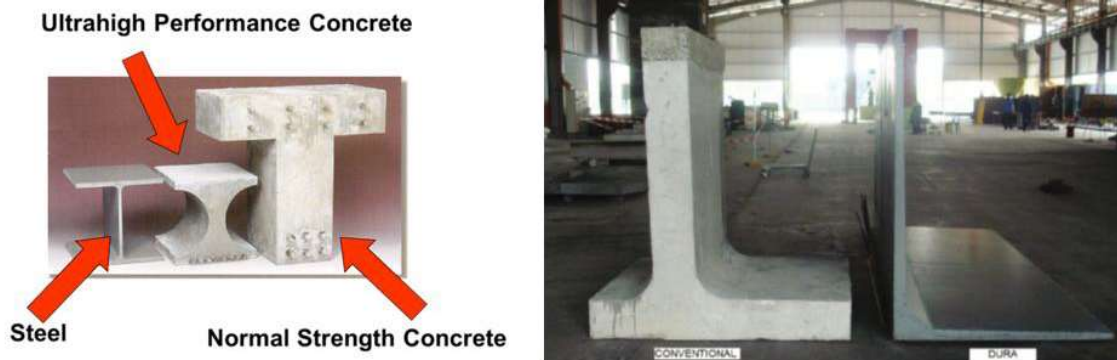
Figure 1-1 Comparison between elements having approximately the same load bearing capacity: (left) steel, UHPC and NC and (right) NC and UHPC.
