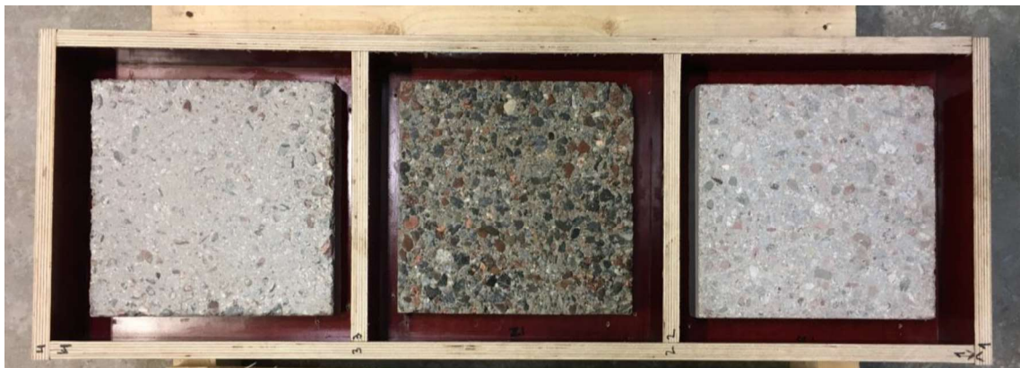
Figure 3-14 Form for UHPC-overlay with different surface treatment of reference concrete. Tests: pull-out
