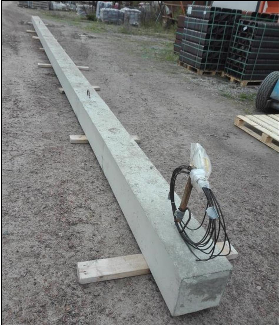
*Figure 3.4.1. The pile used for the experiment. The fiber optic cables that come out from concrete are visible on the top portion of the pile.*
