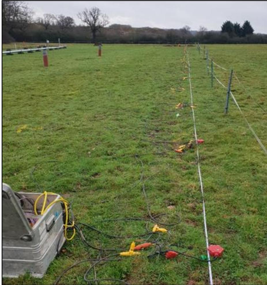
*Figure 2.1.1. Line of 3-axial geophones for the London test*
