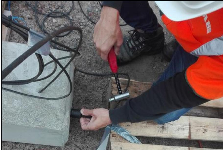
*Figure 3.4.3. Nils Rydén (Peab AB and Lund University) acquires measurements with an accelerometer placed on the smaller side of the pile.*
