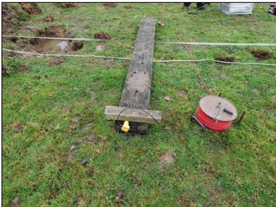
*Figure 2.1.2. Wooden beam as SH source for the London test*
