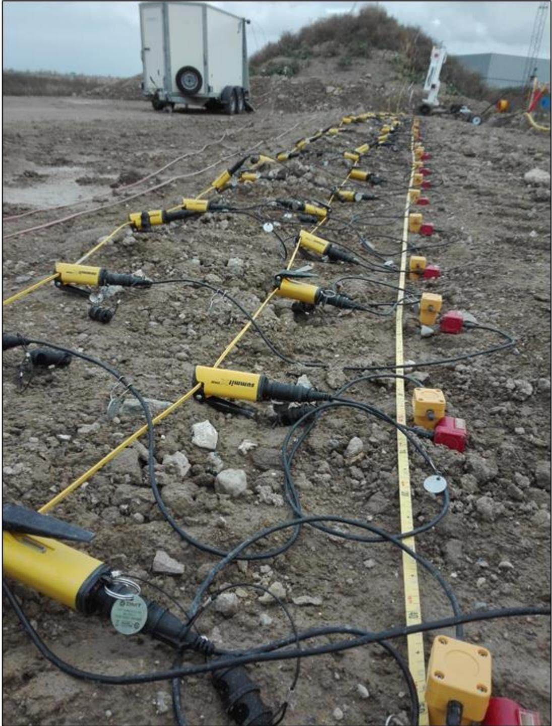
*Figure 3.3.5. Example of geophones layout: Layout 3 with 0.5 m spacing, 4.5 Hz geophones. Yellow receivers are the vertical component geophones, while the red ones are the horizontal (in-line) component geophones.*
