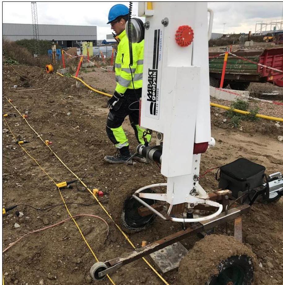
*Figure 2.1.3. ESS100Turbo accelerated weight drop. The Summit X One Remote Units are also visible together with two geophones next to the wheel of the weight drop.*
