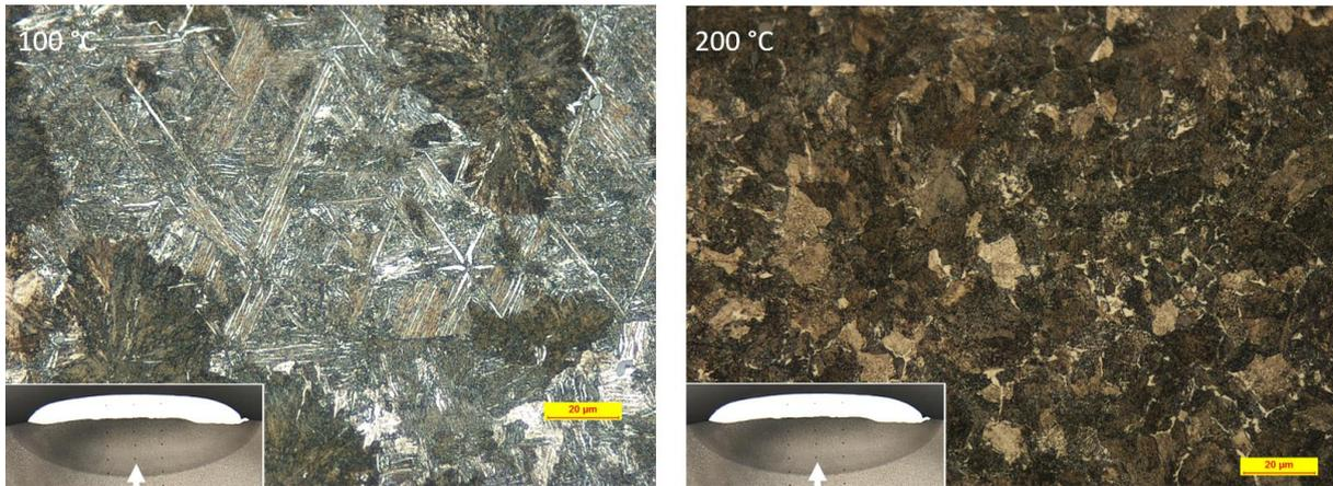
Figure 19: Microstructure lower HAZ. Pre-heating temperature 100°C to the left and 200°C to the right. White arrow illustrates position of image.
