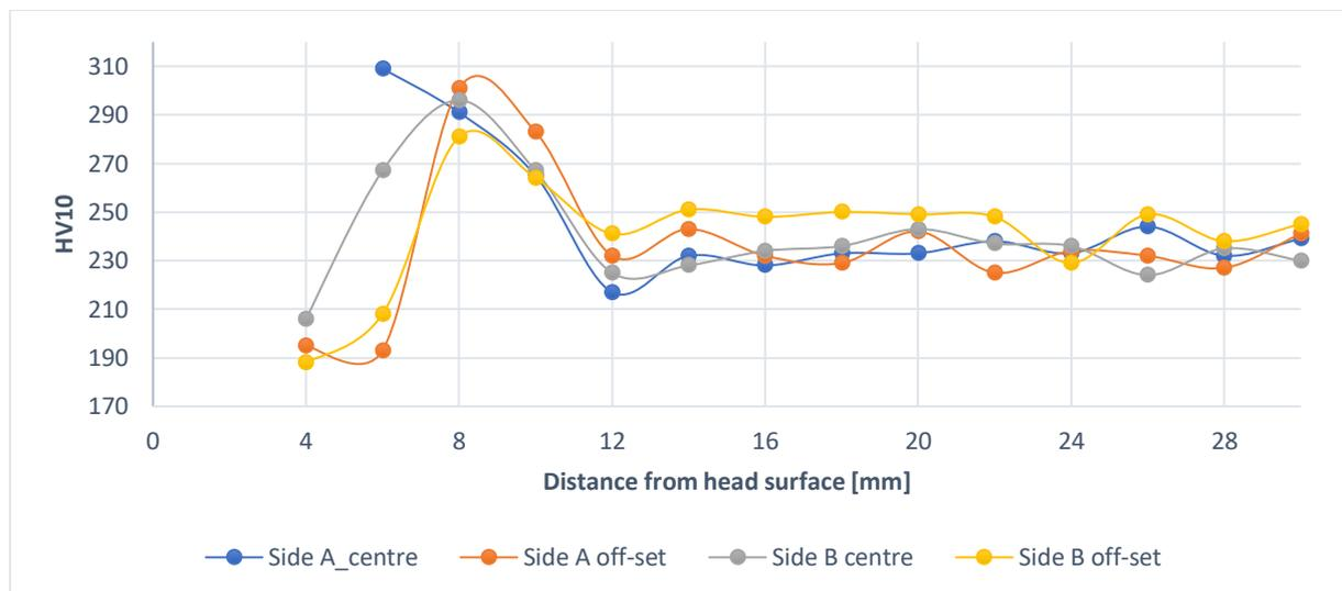
Figure 9: Hardness measurement of electro slag welded rail.
