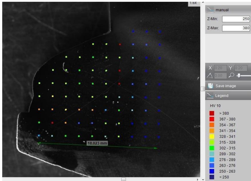
Figure 35, hardness measure of weld C4
