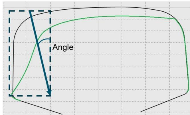
Figure 6, wear profile of a rail with a dotted line illustrating the joint preparation.
