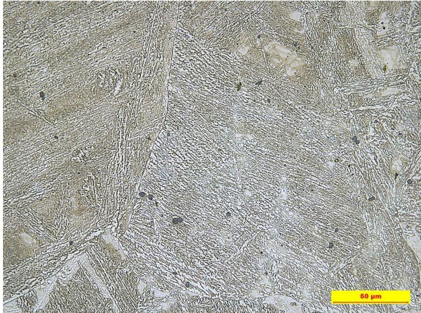
*Figure 14, Microstructure of (first) layer 1 after FCAW welding*
