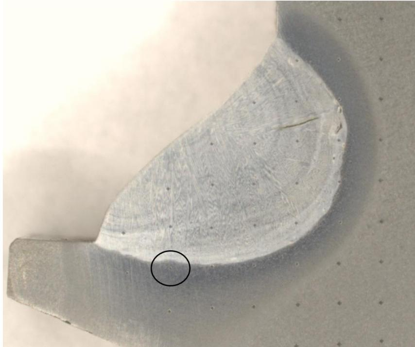
*Figure 26, cross section of weld C2*
