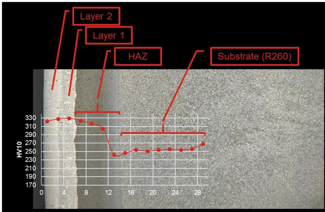
Figure 16, hardness measures from the FCAW welded rail
