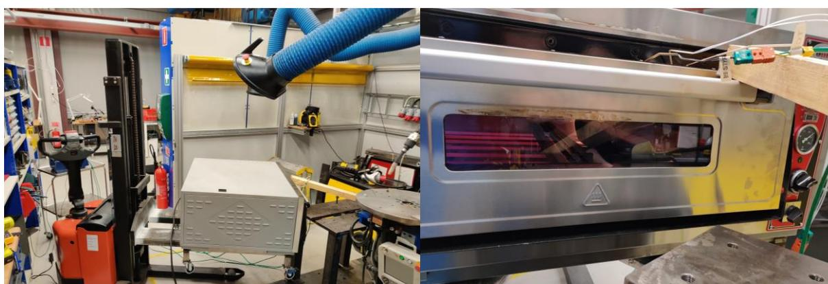
Figure 3, Pizza oven used for preheating.
