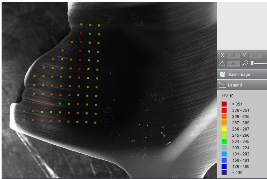
Figure 39, hardness measure of weld C5
