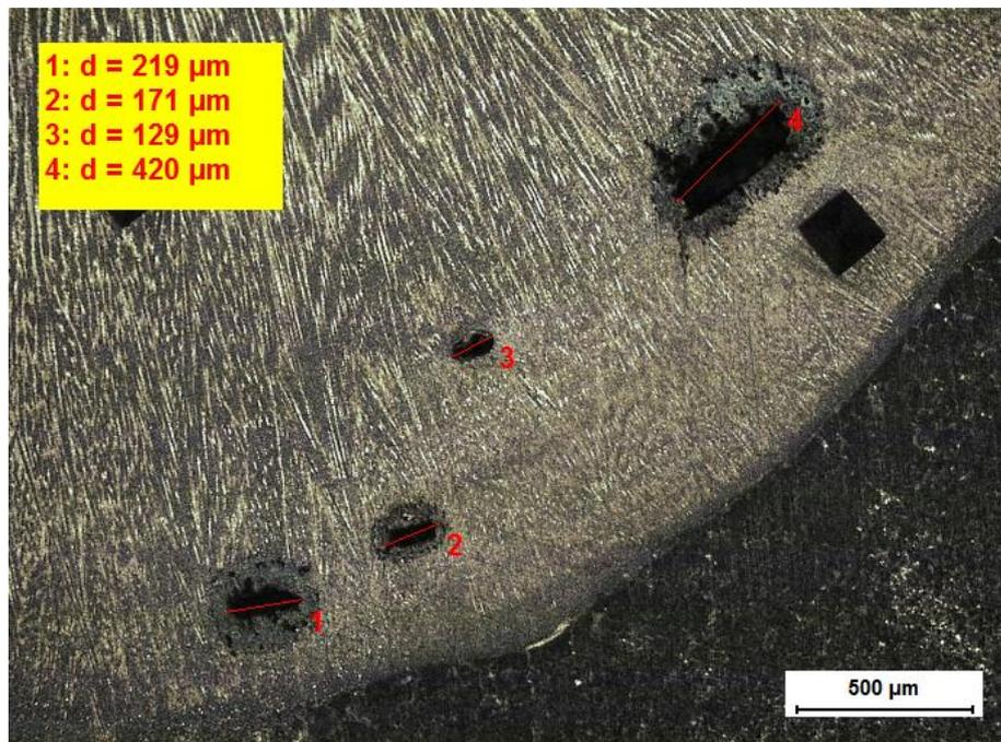
Figure 31, pores in the root of the first weld of C3
