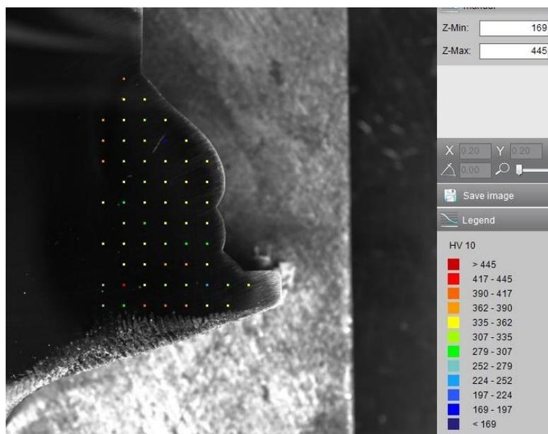
Figure 25, hardness measure of weld C1
