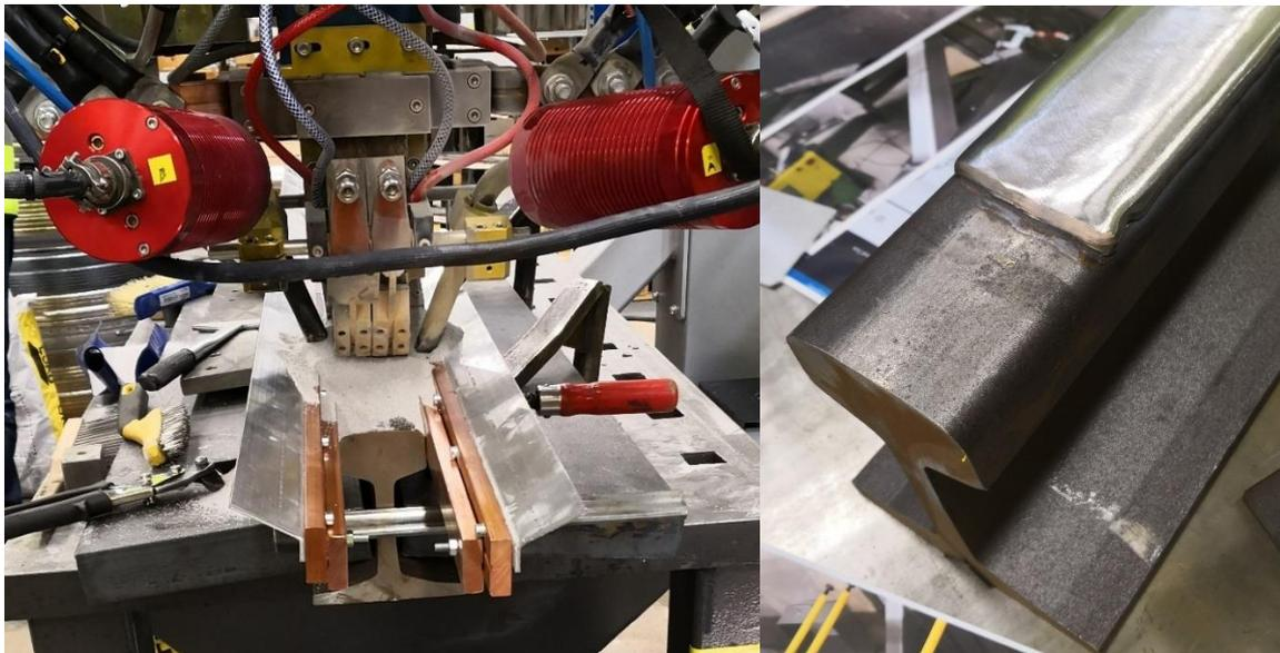
Figure 2, (left) weld setup for ESC welding, (right) finished weld.
