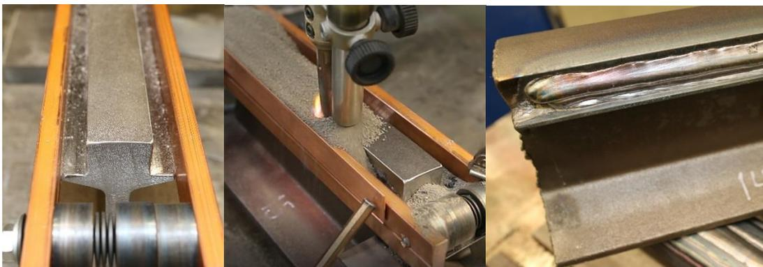
Figure 7, the setup for SAW welding.
