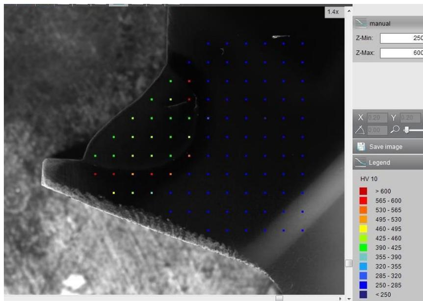
Figure 29, hardness measure of weld C2
