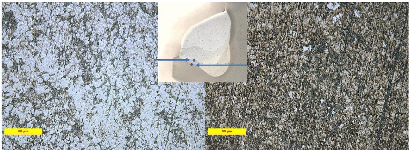
Figure 36: Left- microstructure in first bead, right - microstructure in HAZ close to FL.
