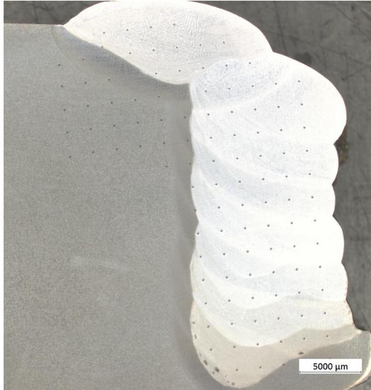
Figure 30, cross section of weld C3
