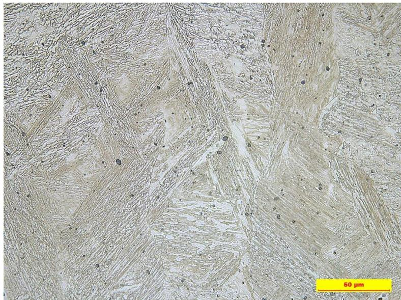
*Figure 15, Microstructure of layer 2 after FCAW welding*
