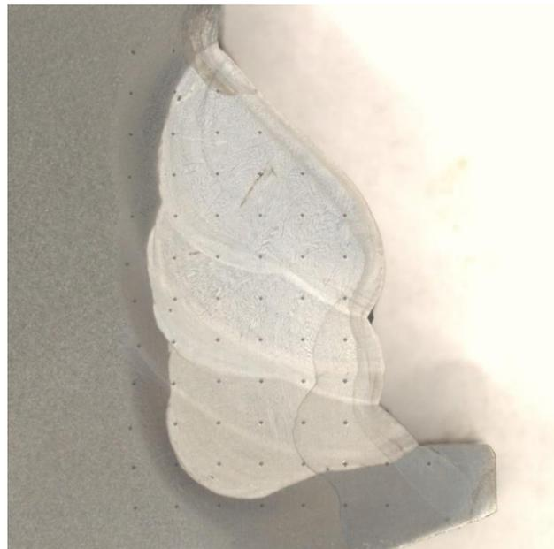
*Figure 23, cross section of weld C1*
