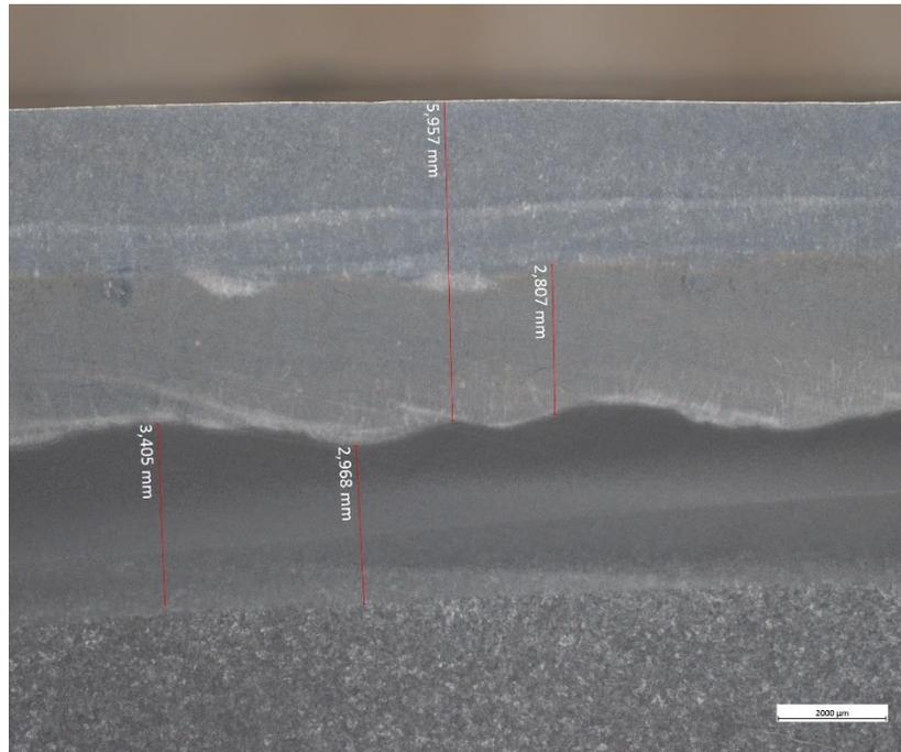
Figure 10, cross section of the middle of the rail.
