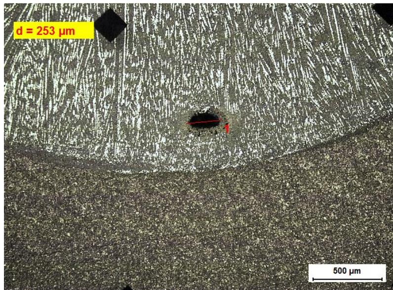
*Figure 38, pore in the root of weld C5*
