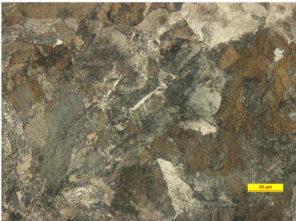
Figure 20: base material 6mm from HAZ boundary.
