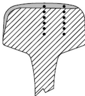
Figure 8: Hardness measurement on cross-section surface
