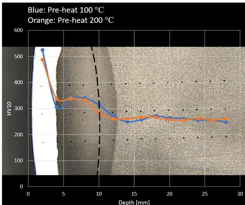
Figure 22: SAW strip mean hardness. Background is cross-section of sample pre-heated to 200 °C. Dashed line is HAZ boundary.
