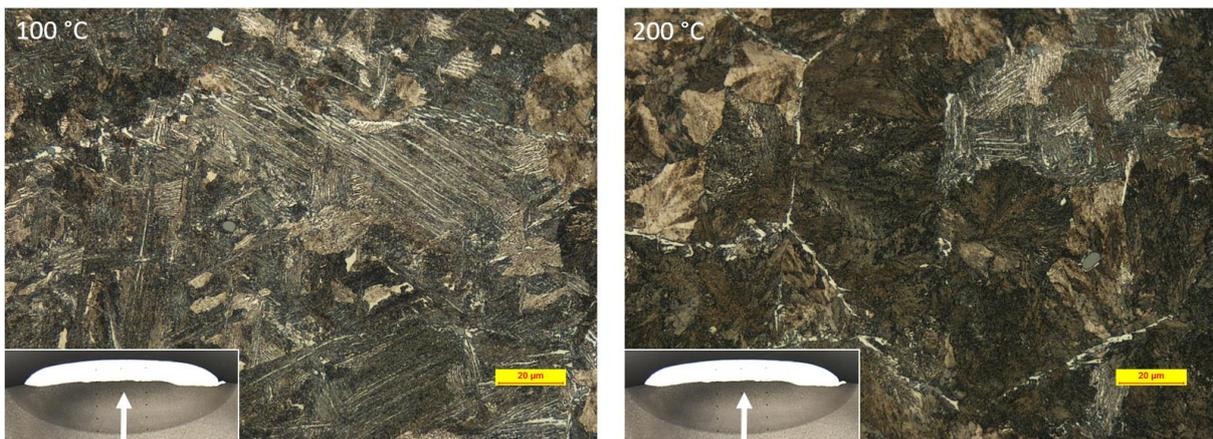
Figure 18: Microstructure of upper HAZ. Pre-heating temperature 100°C to the left and 200°C to the right. White arrow illustrates position of image.
