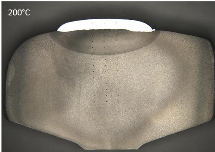
Figure 21: penetration profiles of SAW strip cladded railhead, pre-heated 200°C
