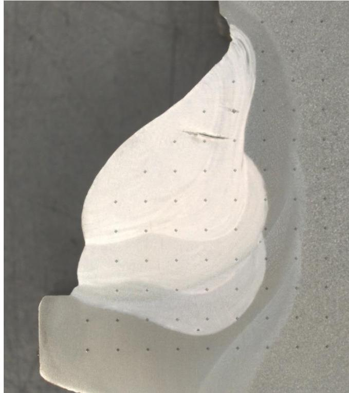
*Figure 37, cross section of weld C5*
