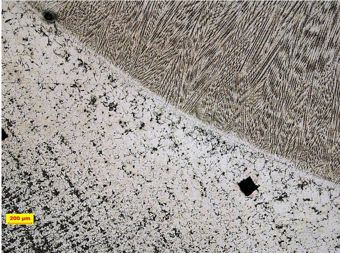
Figure 27: interface between base material and weld metal, with fusion line separating them. The hardness is 565HV10 in the hardness indentation.
