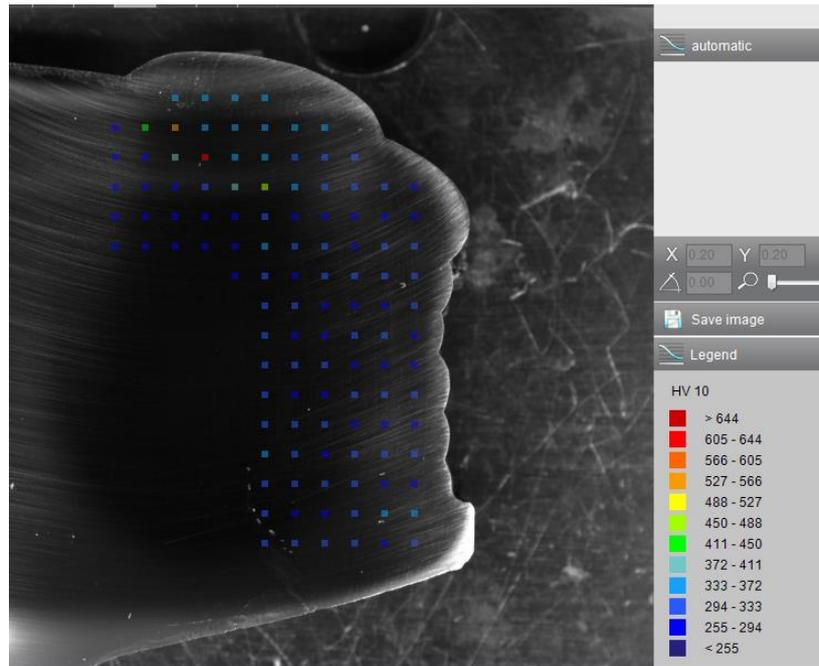
Figure 32, hardness measure of weld C3
