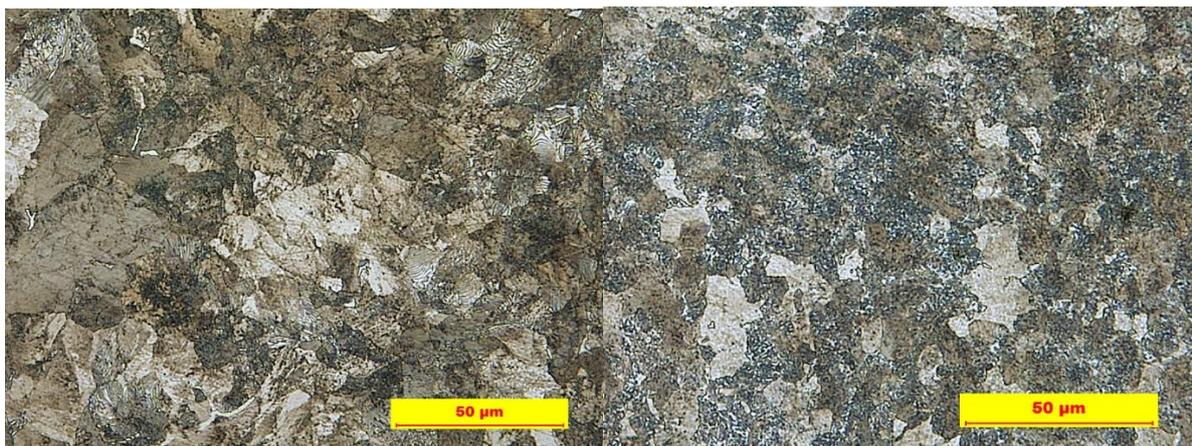
*Figure 13, left, microstructure in the top of the HAZ, right the bottom of the HAZ.*
