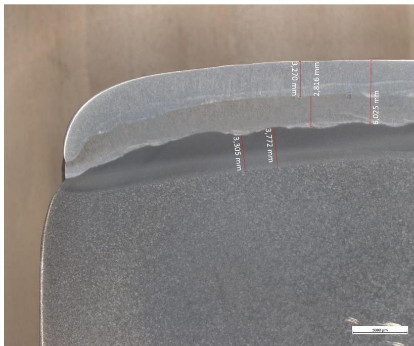
Figure 11, cross section from the edge of the rail.
