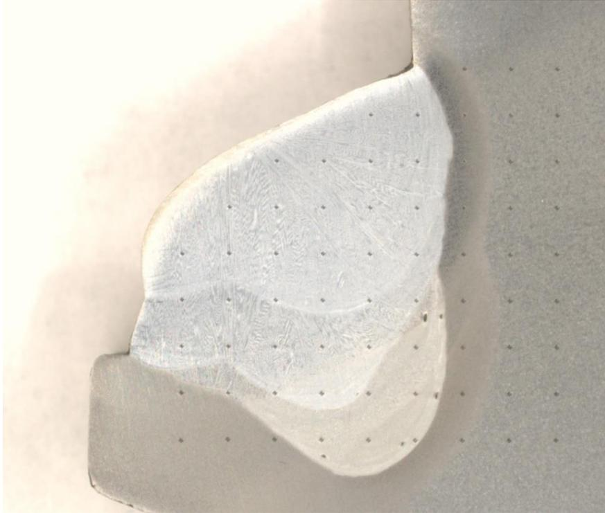
*Figure 33, cross section of weld C4*
