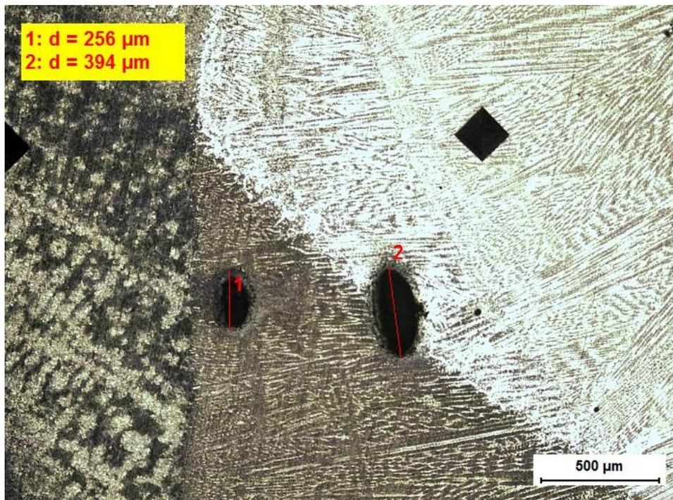
*Figure 34, example of pores in weld C4*
