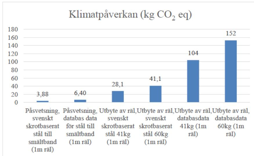
Figure 1: LCA comparing repair and replacing rails in the track [1]
