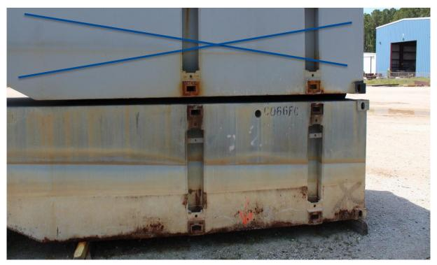
Figure 10. Unit C066FC, probably manufactured during early 1990. The DFT above the 1<sup>st</sup> waterline was about 180  $\mu$ m, between water lines about 90  $\mu$ m, below the 2<sup>nd</sup> water line 30 $\mu$ m. Below the 2<sup>nd</sup> waterline rust and barnacles were found.
