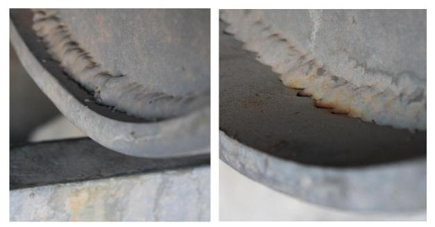
Figure 30. Irregular weld profiles with deep undercuts. To the left: generally, this type of weld was free from corrosion. To the right: a few poor welds had started to rust.
