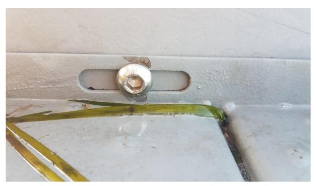
Figure 40. The coating had chipped around this stainless allen bolt. There was however little or no corrosion. One reason for this could be that the silicate binder creates a passivating silicate layer on the steel. Another explanation could be that the coating is protecting the steel cathodically.
