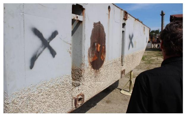
Figure 25. Reference unit coated with 400  $\mu$ m epoxy. Barnacle growth under the waterline. Welds with insufficient pretreatment around the manhole had begun to rust and the coating had started to under rust.
