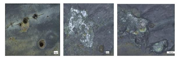
Figure 83. Some pinholes were found in the coating. To the left: pinholes as found. In the middle: The coating was scraped with the edge of a knife, revealing metallic zinc under the surface of the coating. To the right: the scraped surface reacted instantly with copper chloride to form black corrosion products, that indicate corrosion of the metallic zinc.
