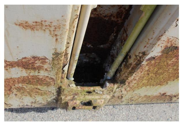
Figure 23. Reference unit coated with 400  $\mu$ m epoxy. Under rusting and flaking was found beneath the waterline.
