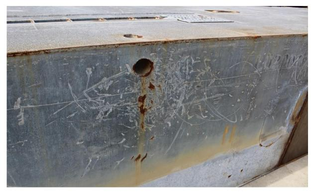
Figure 14. Unit L0 200, a surface subjected to mechanical damage. The coating is relatively resilient towards impact and there was no chipping or flaking around the damaged areas. DFT in the scratches without rust was about  $30 \mu m$ .
