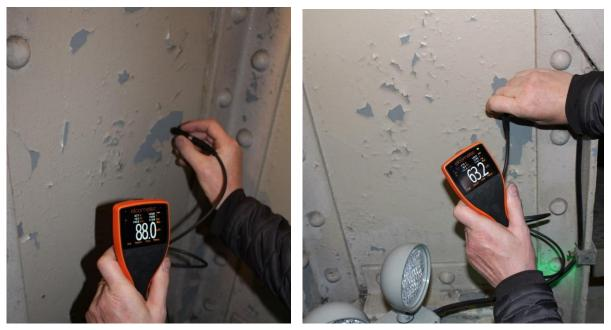
Figure 5. Generally, the film thickness of the silicate coating was between 60-90  $\mu$ m.
