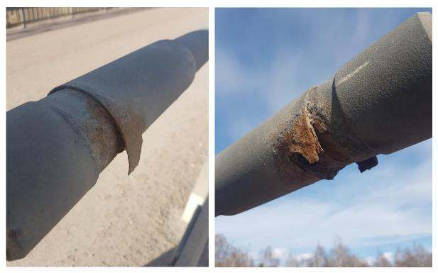
Figure 72. Two examples of crevice corrosion in the expansion joints of the handrail.
