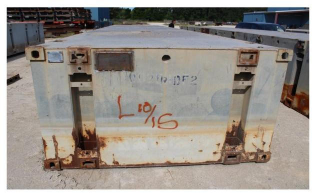
Figure 19. Unit Q0254, probably manufactured during early 2000. The zinc pigment appears to be consumed under the water line and as a result the steel has started rusting, some barnacles were visible. It appears that the coating deteriorates by gradual erosion from the outside and in rather than via flaking and under rusting.
