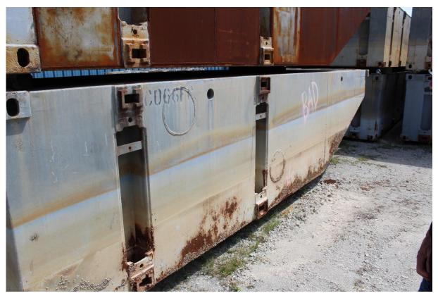
Figure 11. Unit C066FC, the presence of barnacles below the second waterline could be an indication that all zinc has been consumed and as a result, the barnacles can start to grow.
