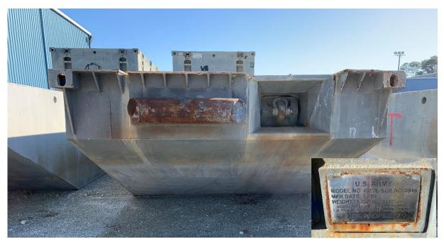
*Figure 8. Unit 0046 with an engraved sign with manufacturing month. This unit was manufactured 29 years ago. The chamfered part of these units is used to drive the modular system onto the seashore*
