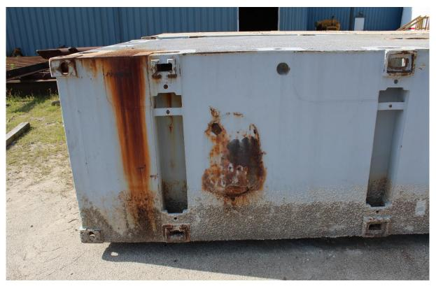
Figure 24. Reference unit coated with epoxy. Corrosion on welds around manhole. Significant growth of barnacles under the waterline.
