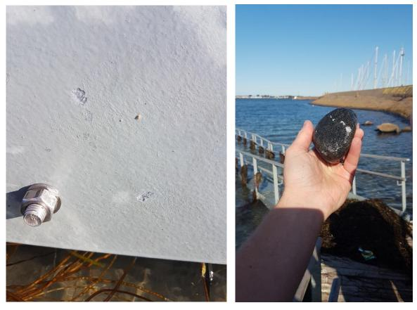
Figure 42. A damage in the coating was introduced by throwing a rock at the outside girder of the ramp. The impacts tended to create indentions in the coating rather than chipping it. Some zinc got stuck on the stone. The DFT in the indentations was about  $40\mu m$ .
