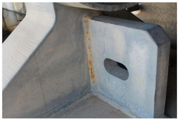
Figure 32. Rust on a weld with adequate smoothness. The premature coating failure on this weld is probably due to an inadequate blasting profile on the weld, which in turn had led to loss of adhesion.
