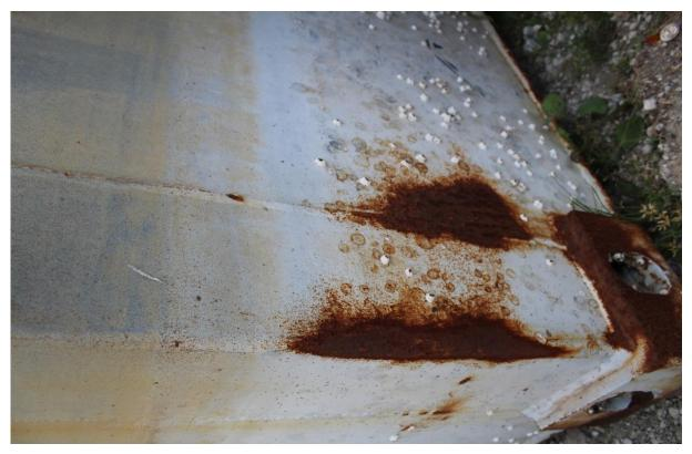
Figure 16. Unit P40 552, DFT was about 90 $\mu$ m above the waterline, DFT was about 30  $\mu$ m below the water line. The antifouling action could possibly be explained by leaching zinc salts. A change of colour in the coating below the water line suggests that all the zinc has been depleted and left a thin silicate coating where the barnacles can grow.
