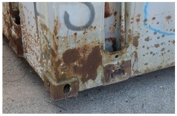
Figure 22. Reference units coated with  $400\mu m$  epoxy. The coating had started to break down under the waterline.
