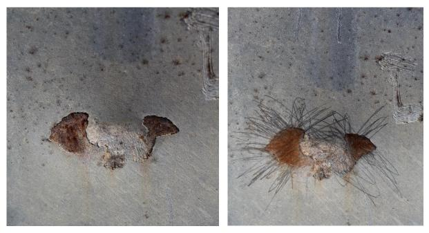
Figure 21. Unit Q0254 to the left: damage after impact. To the right: loose coating was removed with a screwdriver, no rust creep under the intact coating was observed.
