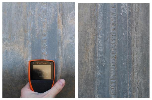
Figure 29. Welds between the two halves of dam gates. No signs of corrosion despite apparent poor pretreatment and low DFT. According to Earl Ramlow who was inspecting the installation of the dam gates, the weld has been laid through the coating and the resulting weld has been ground with a flap disc and painted with a brush to a DFT of about 60µm
