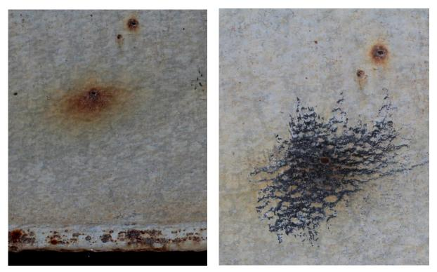
Figure 18. Unit Q155FC, to the left: pinholes and rust discoloration. To the right: The pinhole was abraded with a knife held at 90 degrees to the surface. There was no lateral rust creep from the pinholes, but intact zinc coating was found underneath the discoloration. The pit depth was approximately 2-3 mm.
