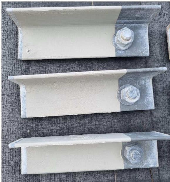
Figure 68 System L, Induragard, no pretreatment
