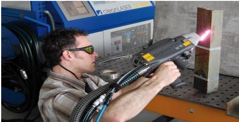
Figure 23. Handheld laser 1000W as depicted at www.agaria.se . Laser nozzle in the foreground and aggregate in the background.
