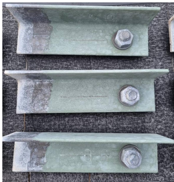
Figure 53 System C, Zn ESI w scribe laser
