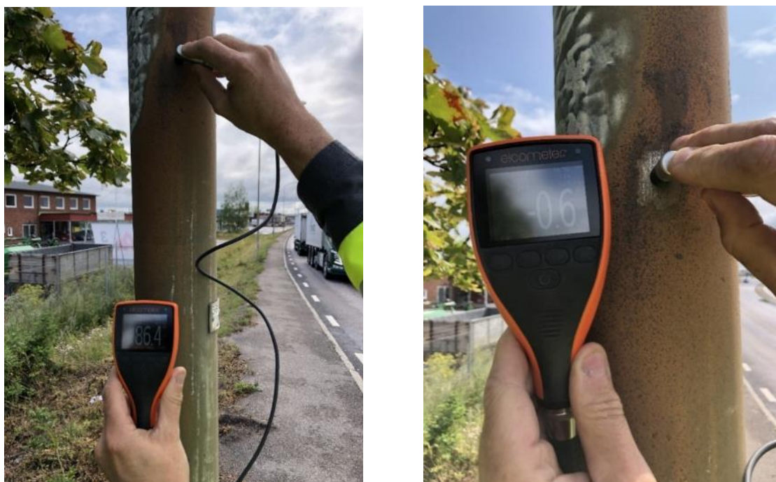
Figure 9. Coating thickness measurement on a lamppost, to the left, measurement as found indicate a thickness of 86 \mu\text{m} . To the right: measurement after scraping gently with a knife held at 90 degree angle, indicate a coating thickness of 0 \mu\text{m} , (the -0.6 \mu\text{m} reading is within the error margin of the instrument).
