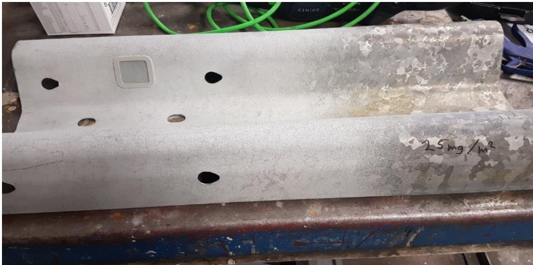
Figure 20. Road fencing that has been partly blasted with slurry blasting. One of the advantages with slurry blasting is that it is relatively easy to wash the surface before blasting, as well as during blasting. Bresle measurements after slurry blasting showed a low salt content on the surface, 25 mg/m 2 .
