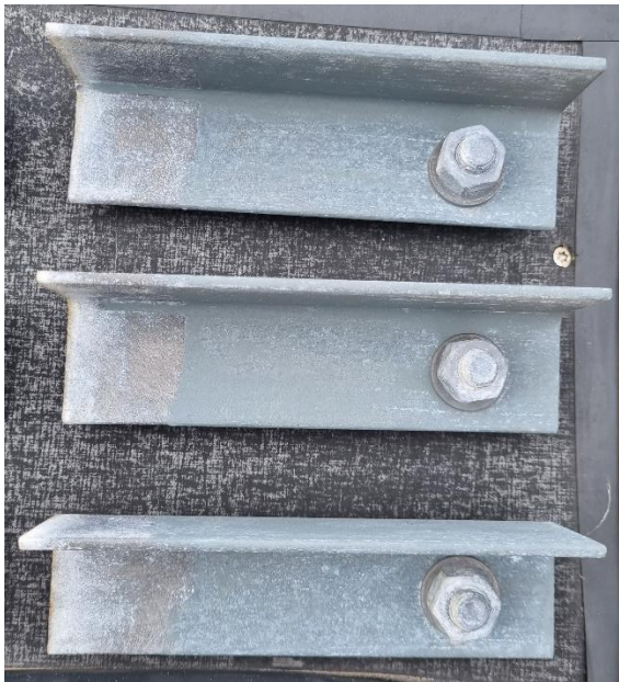
Figure 60 System F, Epoxy (Zn), grinding
