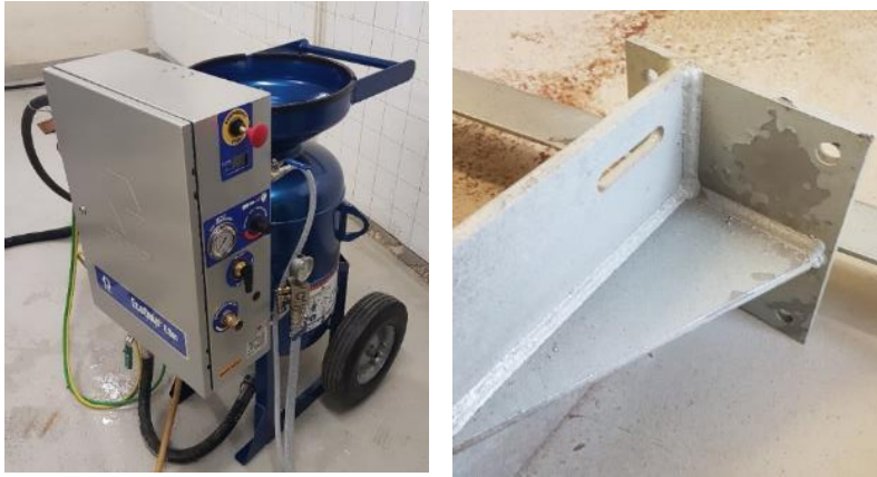
Figure 19. To the left: slurry blasting equipment. To the right: HDG steel structure blasted with slurry blasting equipment, with slurry blasting as with all other blasting techniques it is important to adjust the impact angle and blasting pressure to achieve optimal cleaning. When blasting HDG this is even more important because HDG layers have a tendency to fall off if blasted too hard.
