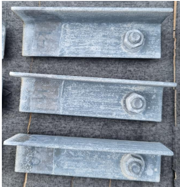
Figure 59 System K, Zinga with scribe, laser
