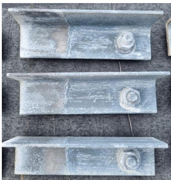
Figure 57 System J, Zinga with scribe, grindnig
