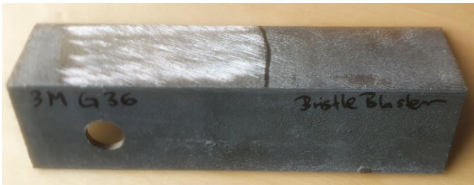
Figure 22. Results after spot repair pretreatment. Hashed grinding to the left of the black indication, bristle blaster to the right.
