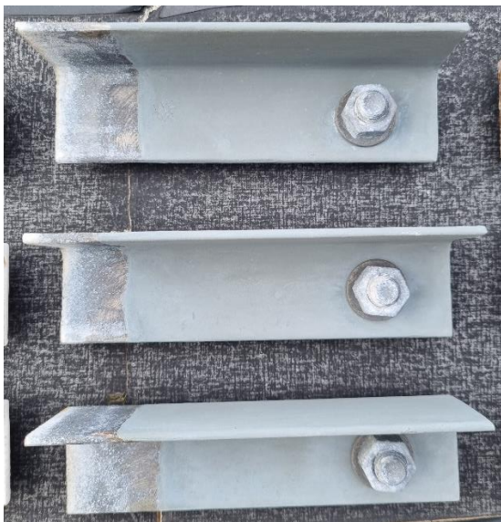
Figure 48 System E, Fontezinc HR, grinding
