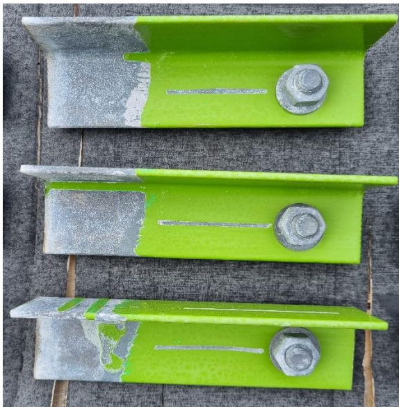
Figure 65 System I, bridge system with scribe, grinding
