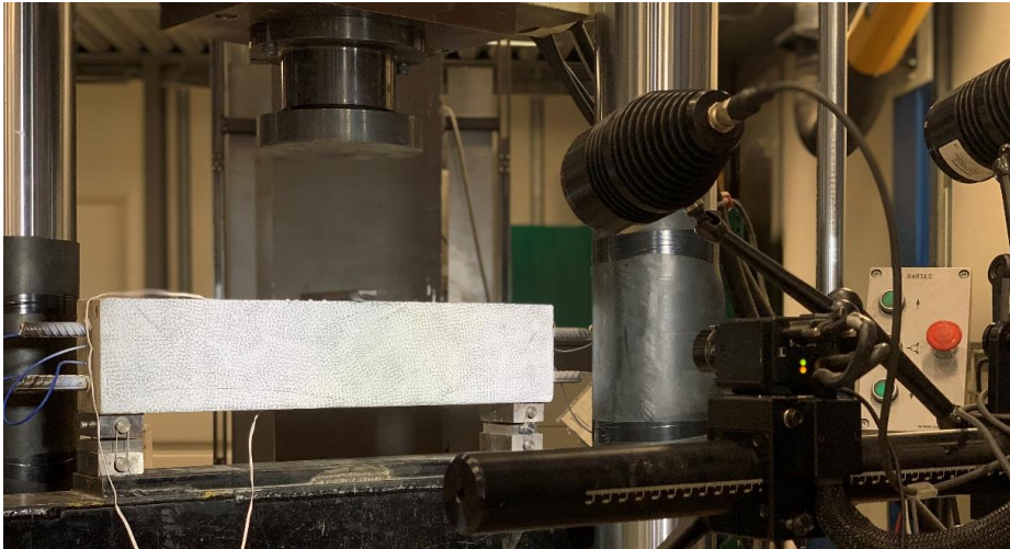
Figure 7: Picture of FOS-beam test, displaying the beam
