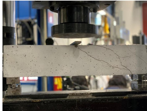
Figure 4. DIC system setup for test cube with speckle pattern after failure (left), cracking on the back side of the beam after failure (right).
