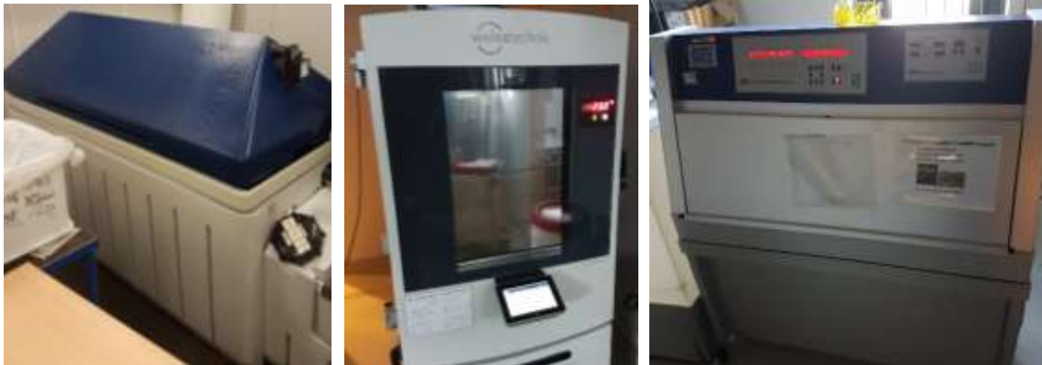
Figure 4. For the ISO 12944-9 protocol, three different cabinets were used, to the right: salt spray chamber, middle: atmospheric cabinet, right: UVA and condense cabinet.
