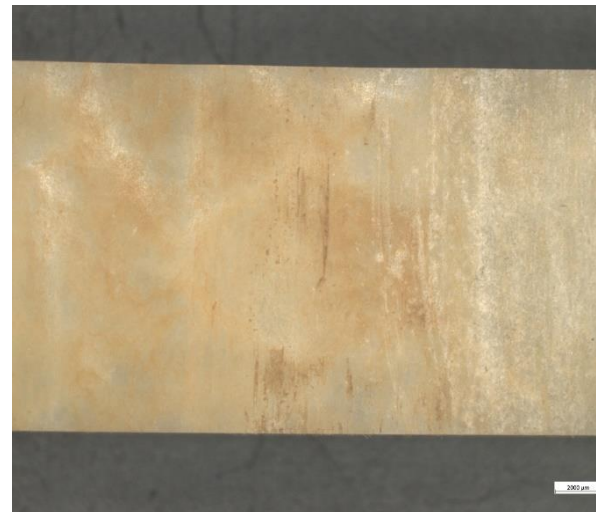
Figure 10. The inside surface of the sample showed good conditions with only surface cracks. The white scalebar is 2 mm.
