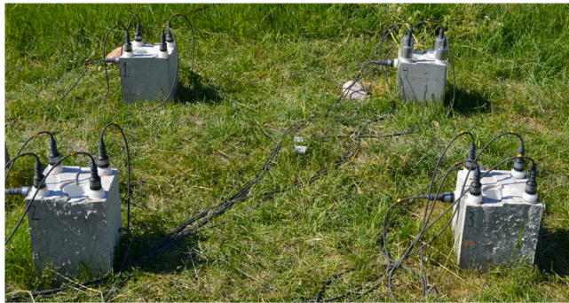
Fig. 5. Measurement setup for the tests on the piles before the casting of the pile cap. The numbering of the piles P1 to P4 are indicated on the side of each pile.
