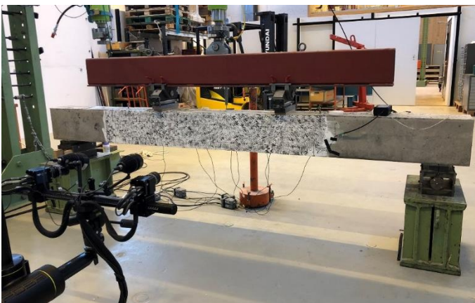
Figure 13 Two point loading test setup for beams (a) with digital image correlation system (b)
