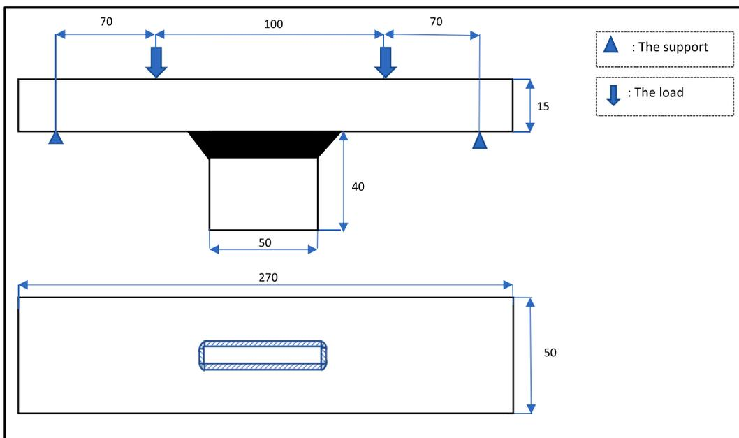
Fig. 10. Dimensions of the longitudinal attachment in mm.
