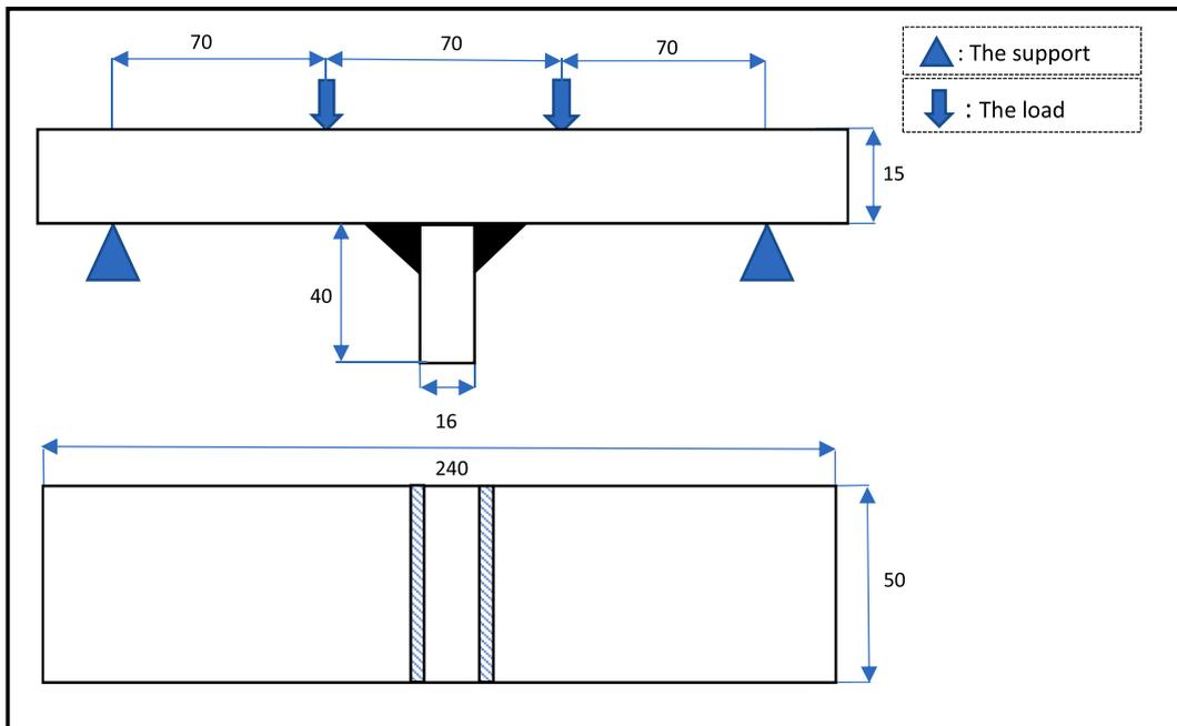
Fig. 9. Dimensions of the transversal attachment in mm.
