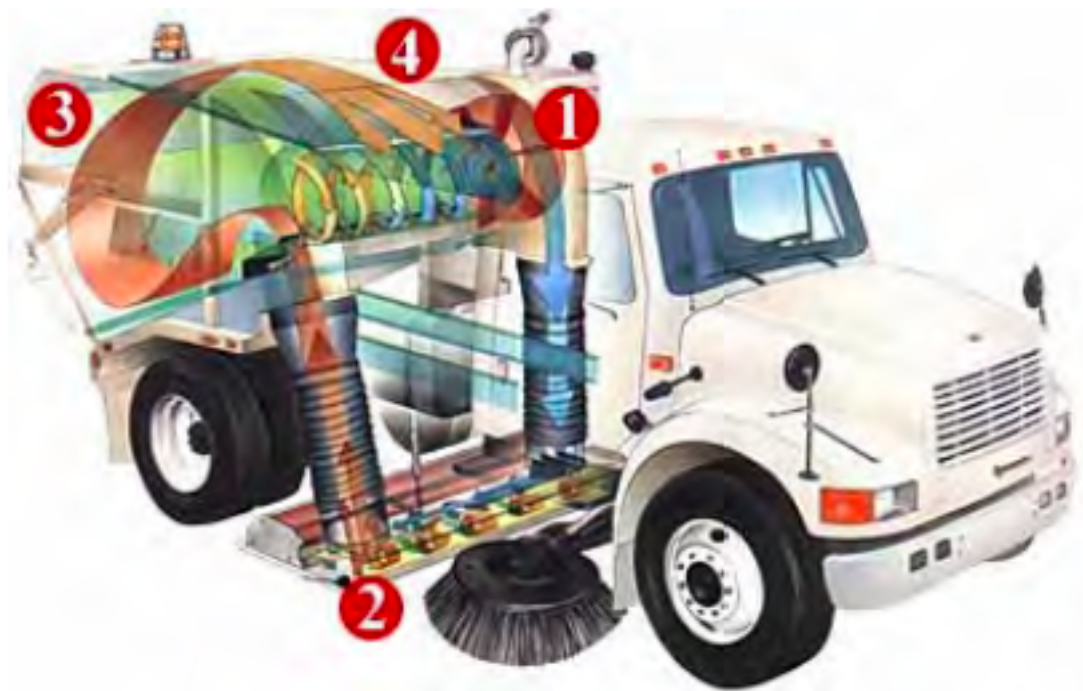
Figure A.1: 1. The regenerative sweeper uses a power air jet, created by a blower wheel. 2. Air blasts down and across onto the pavement and loosens the street sediment. 3. The debris-laden air stream is pulled into the large hopper. There, the larger particles settle on the bottom, while larger objects, such as leaves, paper, cans and rocks are screened, preventing them from entering the centrifugal dust separator. 4. Fine particle are separated because of the centrifugal motion of the air along the curved wall of the chamber. These particles are later transported into the hopper, while the clean air is recycled further (Tymco® 2018).
