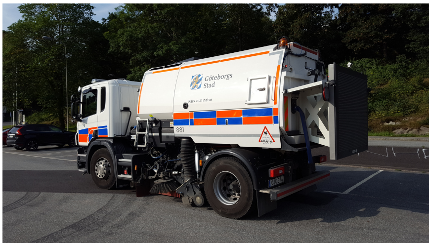
Figure 3.3: Road sweeper VTJB651, produced by Johnston Beam. The brushes were made of steel.
