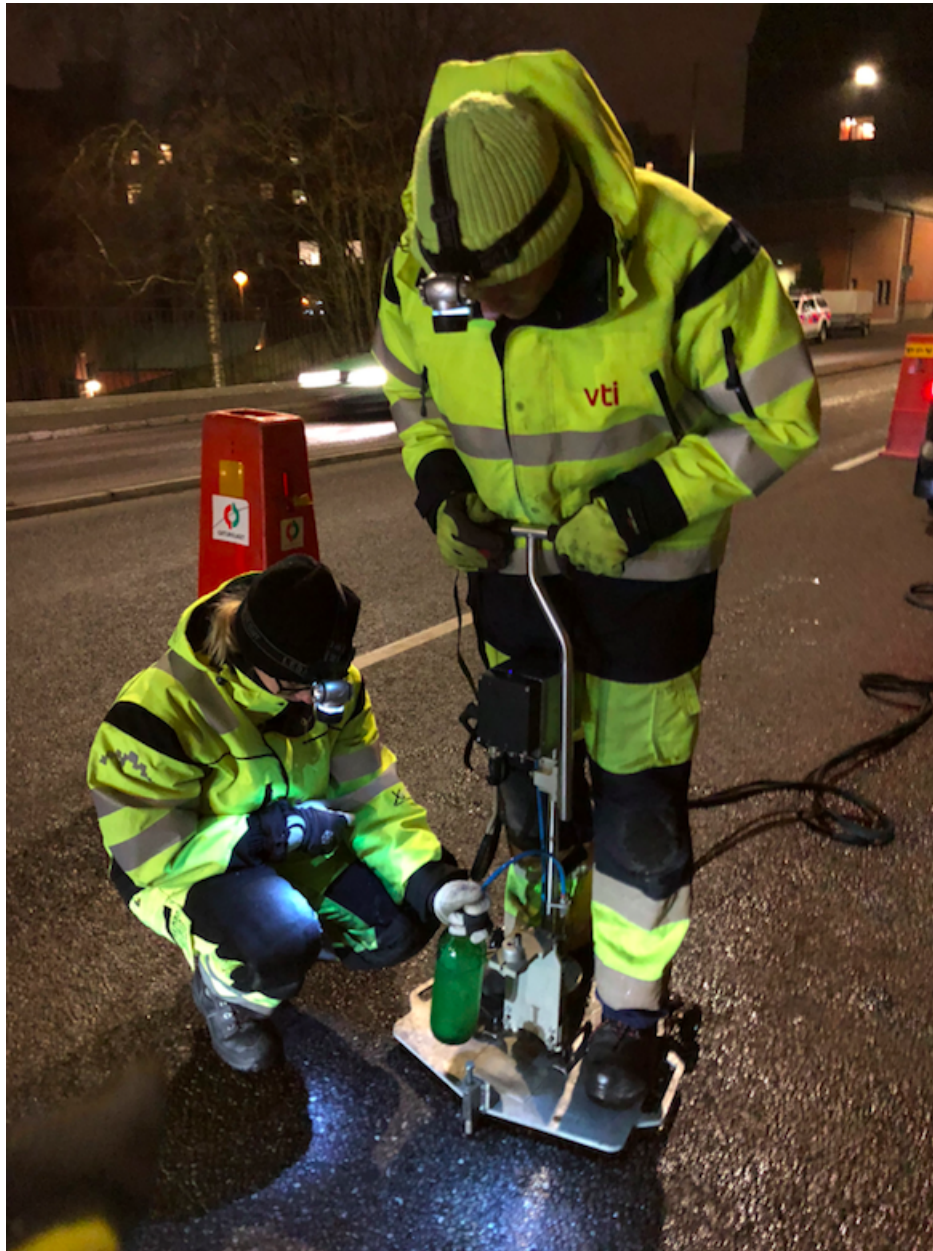
Figure A.3: The sampling of street sediment at the Sahlgrenska catchment area with the WDS during 2018-03-26.
