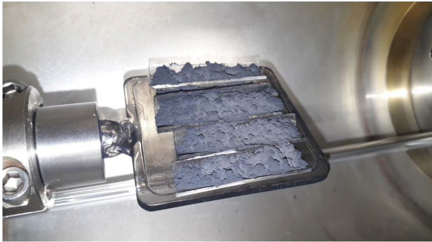
Figure 6. Arrangement of the holders for the synthesis of CNF on cement in the CVD reactor. The darker visible powder is cement covered with CNFs.
