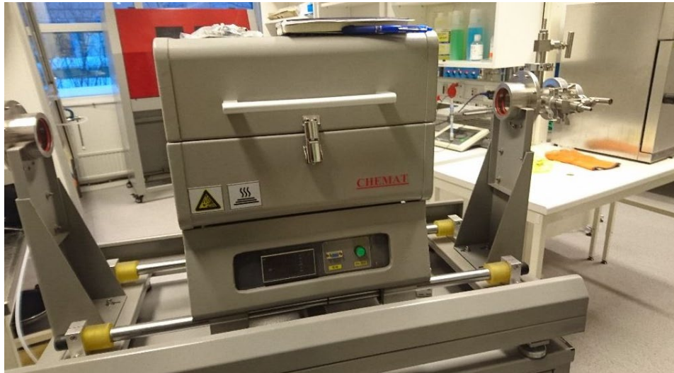
Figure 3. The CVD reactor which was installed for the project but which did not reach a full operational capacity during the project.
