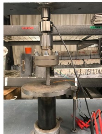
Figure 16. The actual used experimental setup to determine the sensitivity of the produced mortars incorporating various amount of the smart cement to the applied strain and stresses.
