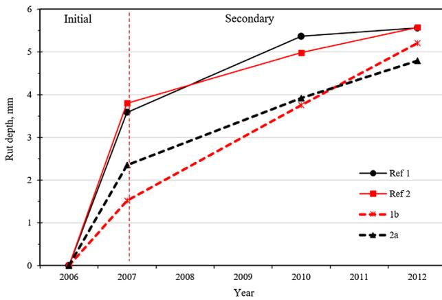
Figure 16. Impact of ageing on modified and unmodified mixes at initial and secondary zones.
