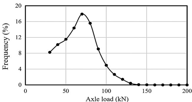
**Figure 18.** Axle load spectra of the selected WIM station.
