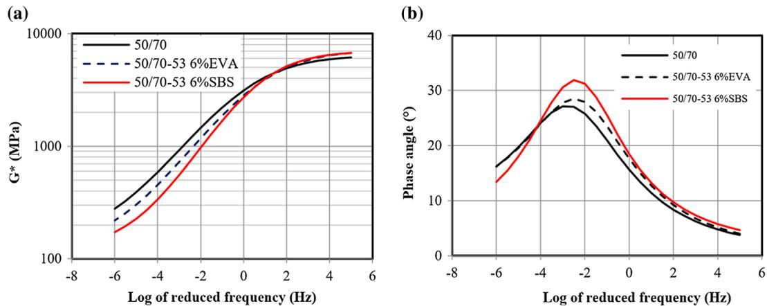
Figure 4. Master curves of (a) Dynamic shear modulus, (b) Phase angle of the binder course mixes ABb 22 with different binders at a reference temperature of 10 °C.
