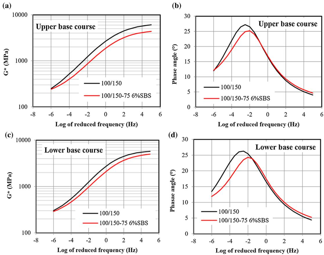
Figure 5. Master curves of (a) Shear modulus of upper base course, (b) Phase angle of upper base course mixes, (c) Shear modulus of lower base course and (d) Phase angle of lower base course, at a reference temperature of 10 °C.
