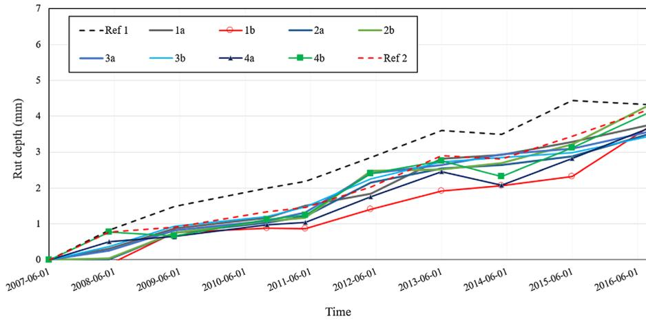
Figure 15. Average rut development in the left wheel track from RST measurements.
