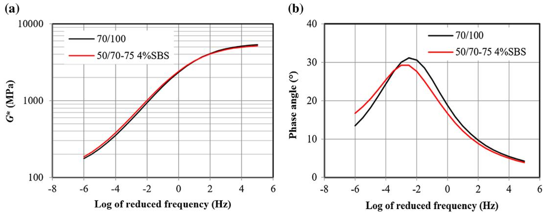
Figure 3. Master curves of (a) Dynamic shear modulus, (b) Phase angle of the surface course mixes SMA 16 with different binders at a reference temperature of 10 °C.
