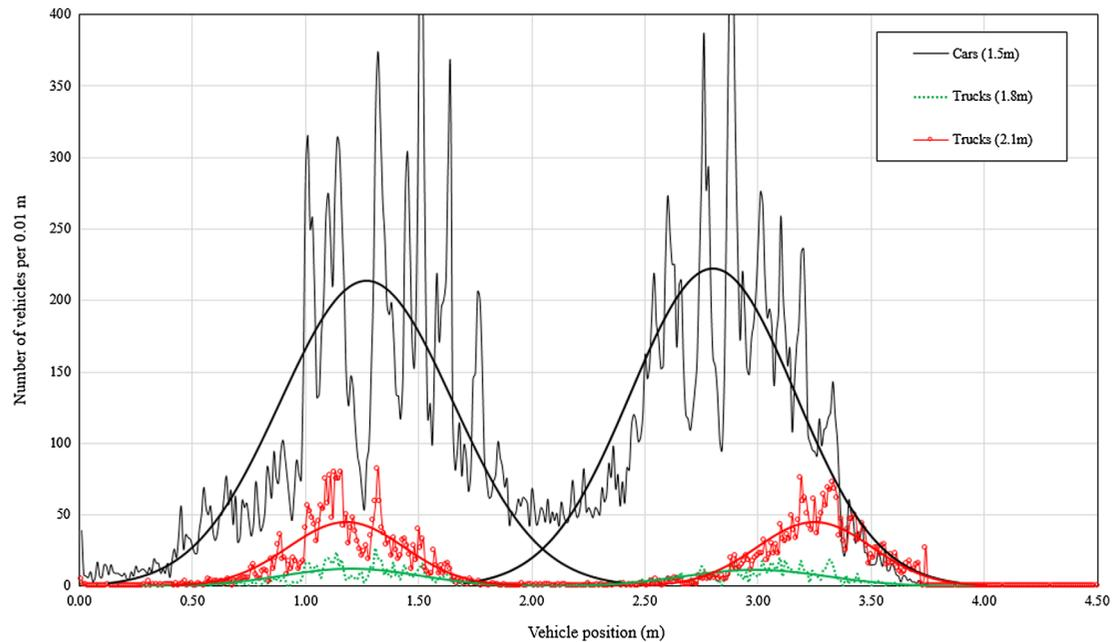
Figure 14. Distribution of lateral position of traffic at the test road motorway E6.
