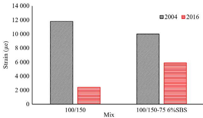
Figure 9. RLCT creep strain of base course mixes from 2004 and 2016.
