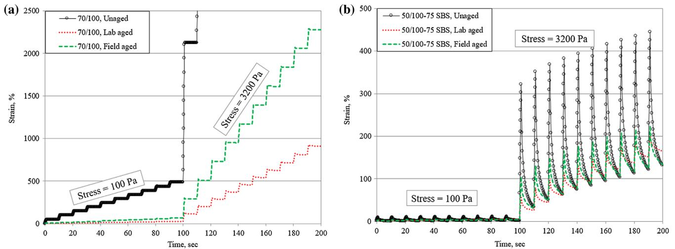
Figure 11. Examples of MSCR test at 60 °C for unmodified and SBS-modified binders.
