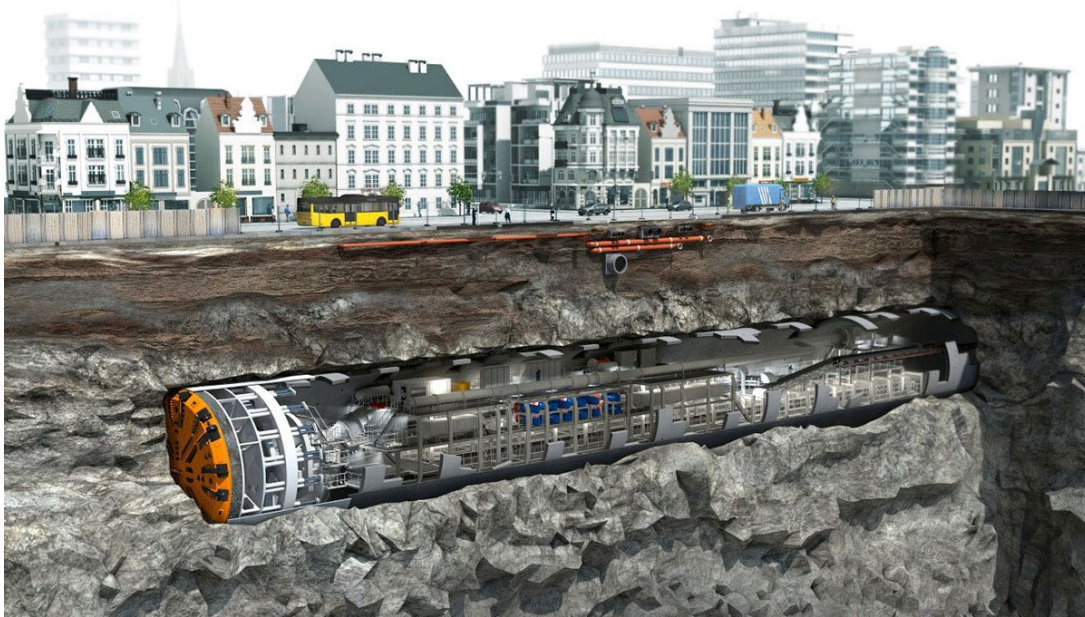
Figure 5 A tunnel boring machine (TBM) in action. The system excavates and simultaneously applies the tunnel lining (from https://www.behance.net/gallery/20377183/ixtract-tunnel-boring-machine-TBM ).
