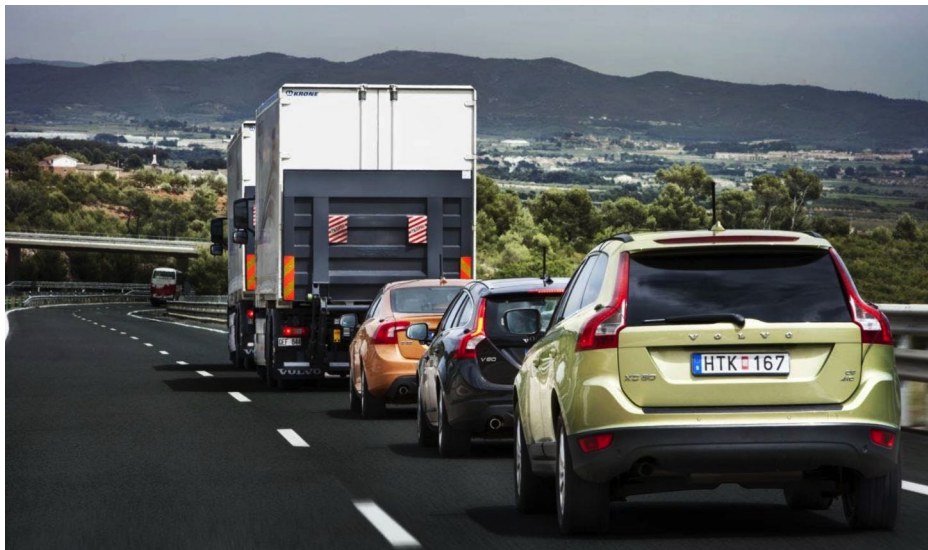
Figure 11 SARTRE project tested platooning on a motorway
