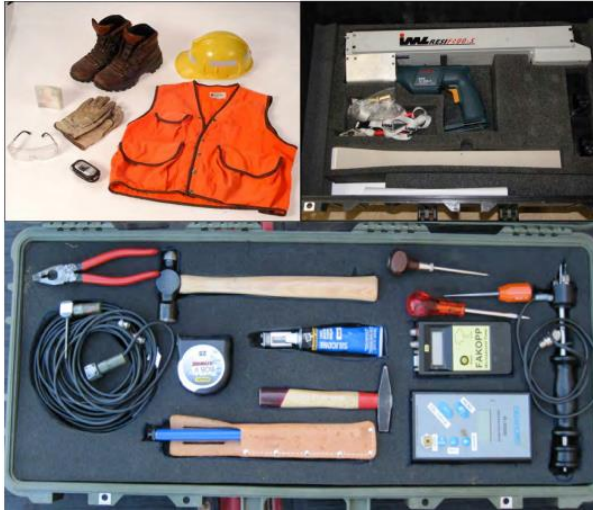
Figure 11 Inspection equipment used for inspection of timber bridges (Brashaw et al. 2014).
