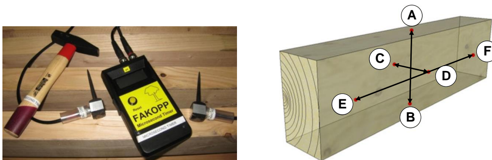
Figure 12 Measurements in different directions (A-B, C-D and E-F) to localise the extent of the damage/deterioration adopted from Dackermann et al. (2014).
