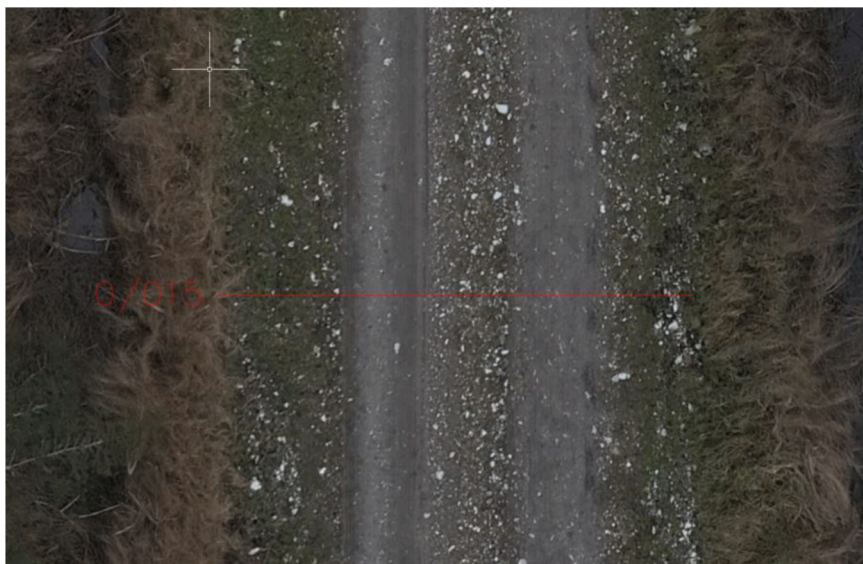
Fig. 2. An Orthophoto taken during the gravel road profiling for visual inspection and interpretation.
