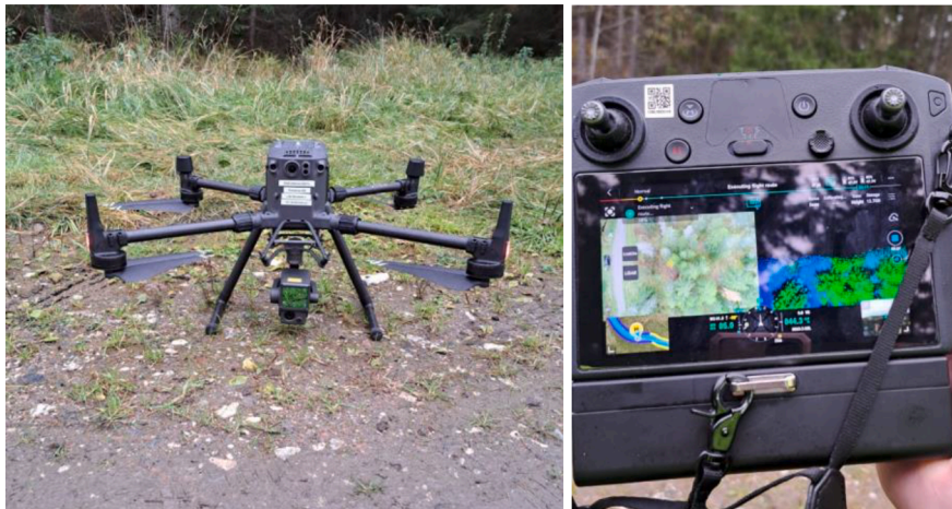
Fig. 1. The DJI M300 Drone with RTK used in the project, photo by Dina Kuttah.
