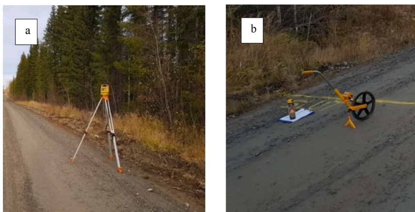
Fig. 3. (a) The rotary laser level, (b) the distance measuring wheel used in the study.
